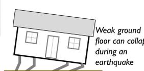
Weak ground floor can collapse during an earthquake
